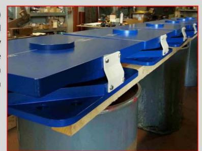
They have a rigid behavior transmitting the loads in all the directions (fixed bearings KBF) or allowing the movement along one direction (sliding guided bearings KBU) or in all the plane directions (free sliding bearings KBM).
