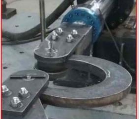
Dissipative bracings: similar to the hysteretic restraints but with axial behavior, therefore suitable when applied as bracings in buildings retrofit where more resistance is required in the static condition but energy dissipation in the seismic one.
